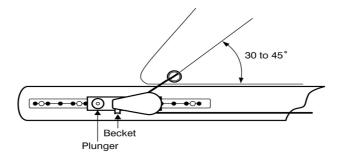
Position the sliders on the track ensuring the plunger end of the slide is aft and the becket on this slide is facing down (this may need to be adjusted depending on whether it is fitted on port or starboard side of the boom. The eye will rotate but may require the use of pliers to carry out this operation).
