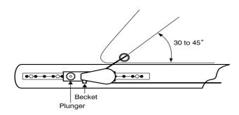
Lower the main Halyard to the correct position for reefing, mark the Halyard at the position of the cleat with permanent marker (reef position 1 + 2).
