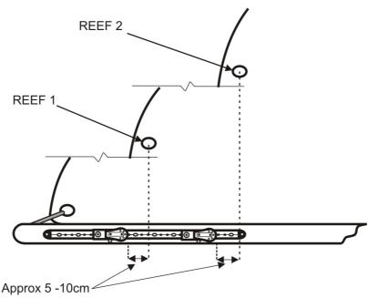
The position of the sliders on the track can be adjusted during a sail trial. The two plastic end caps can now be fitted, ensuring they locate over the end on the track. (This is a push fit) use the centre punch to mark position then remove before drilling and tapping as previously stated.
